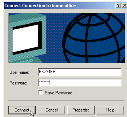
Figure 339. Starting the L2TP tunnel on the Windows 2000 client
