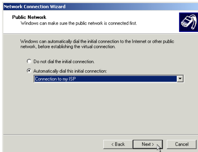
Figure 330. Automatically dial PPP connection to ISP when starting the L2TP connection
