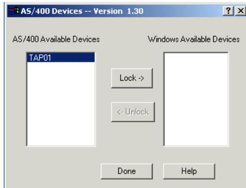
Figure 82. Locking an iSeries tape device to Windows 2000
