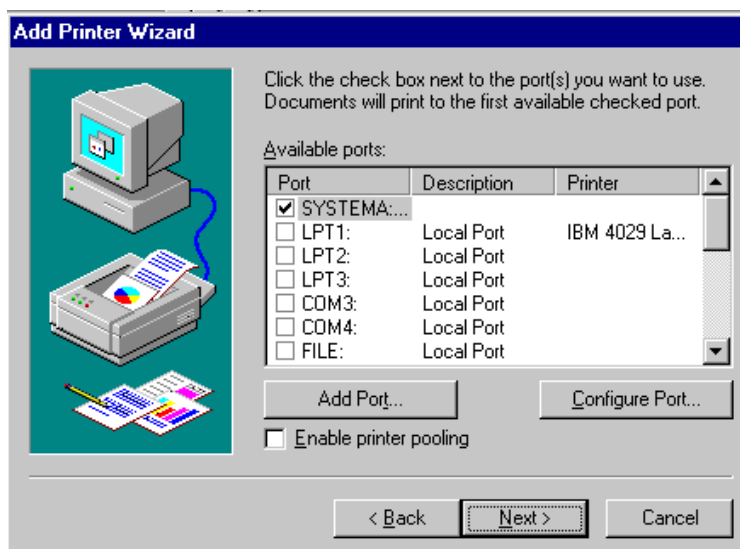
Figure 146. LPD Added as a New Port
