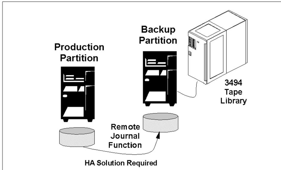
Figure 83. Using Remote Journal Function for 24-by-7 Database Availability
