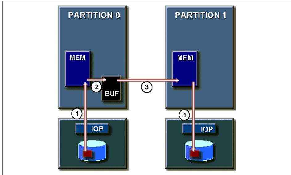
Figure 65. Read Request Using Virtual OptiConnect
