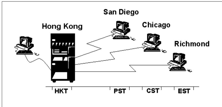
Figure 5. Different Time Zones on One AS/400 System
