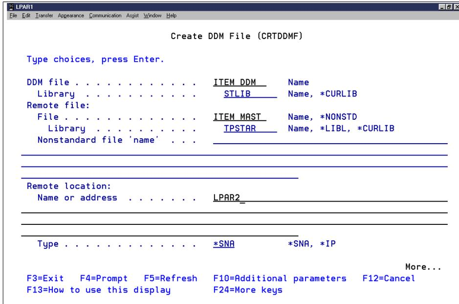
Figure 66. Creating a DDM File to Use OptiConnect (Part 1 of 2)
