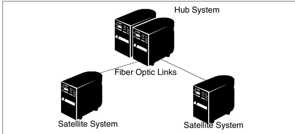
Figure 62. OptiConnect/400 Concept
