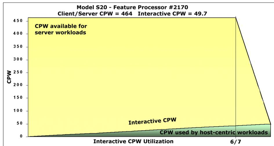
Figure 35. Interactive CPW Utilization — Model S20
