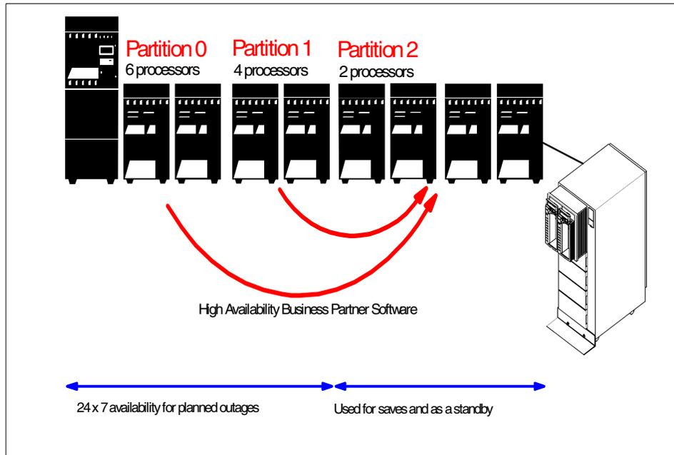
Figure 13. Saving from a Second Copy of the Data
