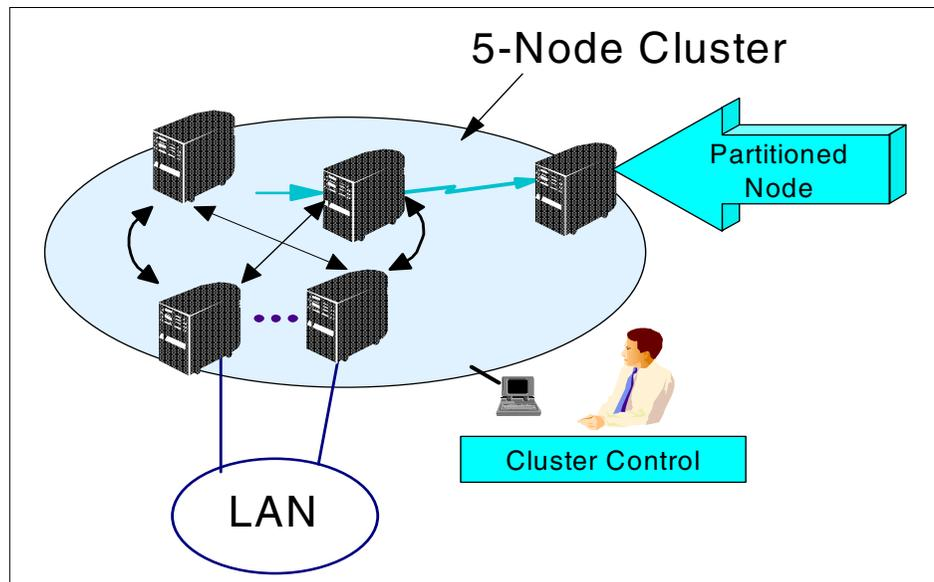
Figure 10. Clustered Configuration with a Partitioned Node
