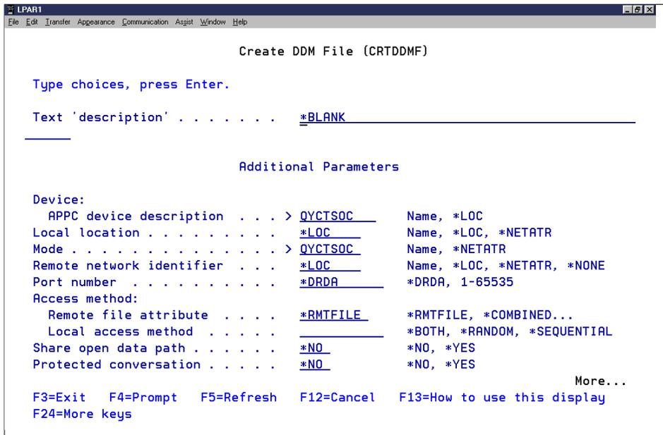
Figure 67. Creating a DDM File to Use OptiConnect (Part 2 of 2)
