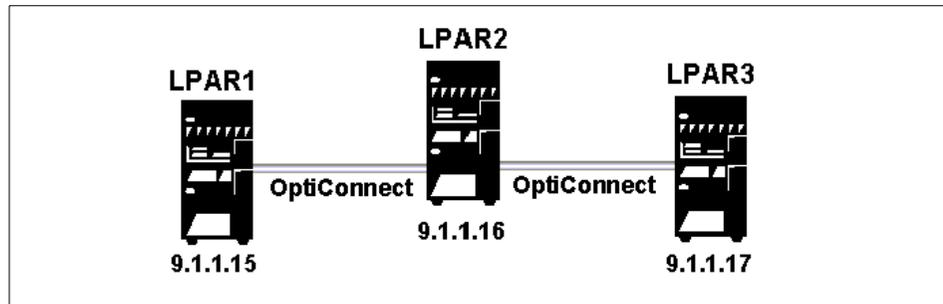
Figure 75. Configuration of the OptiConnect Interface — LAN Version
